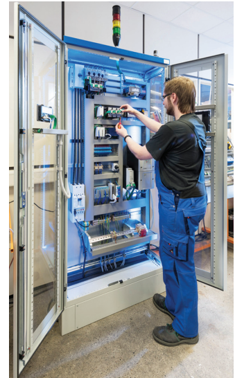
LS Automation uses a cabinet prototype to demonstrate the technical possibilities for constructing and monitoring energy-efficient systems and preparing for ISO 50001, with control technology such as the XV-300, innovative drive technology from the PowerXL range, energy measurement and monitoring based on NZM, BreakerVisu and XMC measuring modules.
