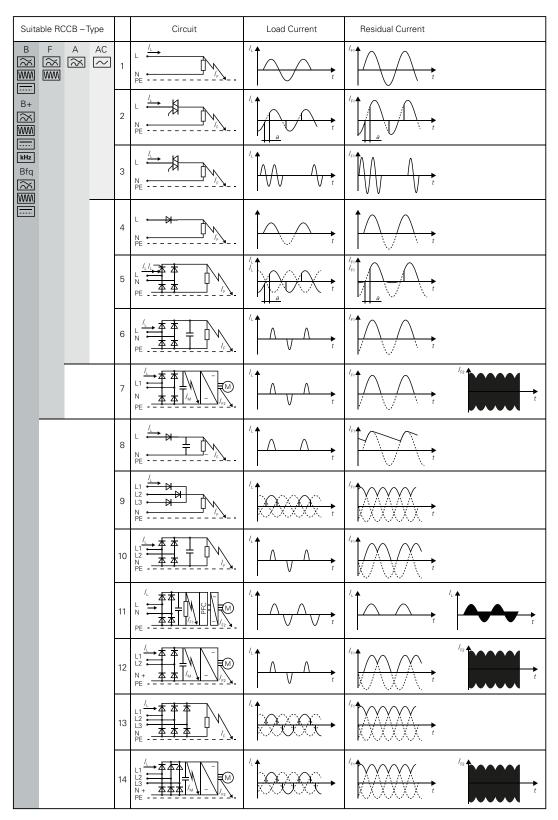
The table shows the possible residual current wave forms and the suitable RCDs.
