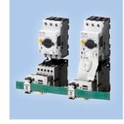
The two-component motor starter, made up of a DILM contactor and a PKZ motor-protective circuit-breaker, is rated for rated operational currents of up to 15 A and features plug-in terminals that make it easy to replace components. Moreover, motor starters rated for currents of up to 32 A can be quickly assembled without any errors by using assembly connectors.
