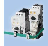
The PKE is a motor-protective and system-protective circuit breaker with modular trip blocks and an electronically implemented overload protection feature. The two component motor starter, made up of a DILM contactor and a PKE motor-protective circuit breaker, is rated for rated operational currents of up to 15 A and features plug-in terminals that make it easy to replace components.
