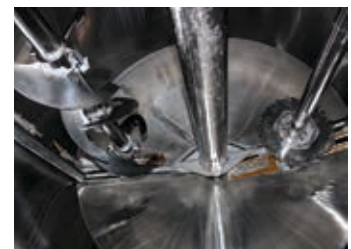
In the mixing vat: The Eaton variable frequency drive controls the speed of the dissolver (right), which breaks up the solid particles in the primary product. The mixer (left) and scraper (middle) slowly move with it (Source: Dinova)
