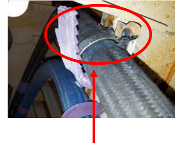
Abrasion location at clamp interface
