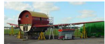
Full size distribution test rig
