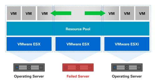
IPM helps maintain business continuity during power failures by triggering an automatic migration of virtual machines to unaffected parts of the network or to an off-site backup facility, co-location data center or cloud computing infrastructure.
