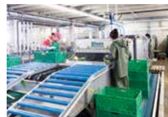
The system for the Pfälzer Renner vegetable production plant is capable of cleaning and cutting different vegetables, depending on the degree of soiling
