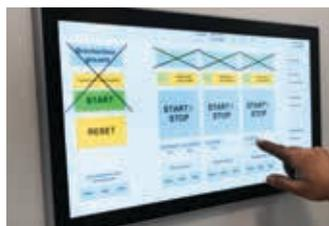
Visualization at the control panel is based on a modern touch panel with capacitive multi-touch technology.
