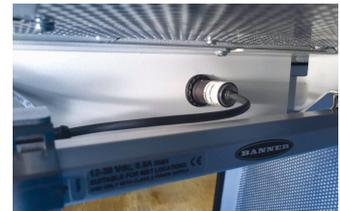
With protection class IP67/IP69K on the front panel and the sealed cable and protection class IP65 on the rear, the illuminated pushbutton is fully protected against dust
