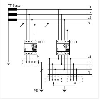
Fig. 8: Residual current protective devices in different earthing systems
