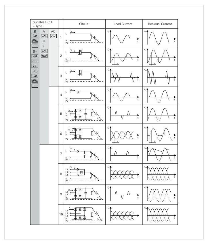
Table 2: Possible residual current waveforms and suitable residual current protective devices (Source: EN 61800-5-1 standard)
