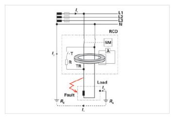
Fig. 2: RCD principle of operation
