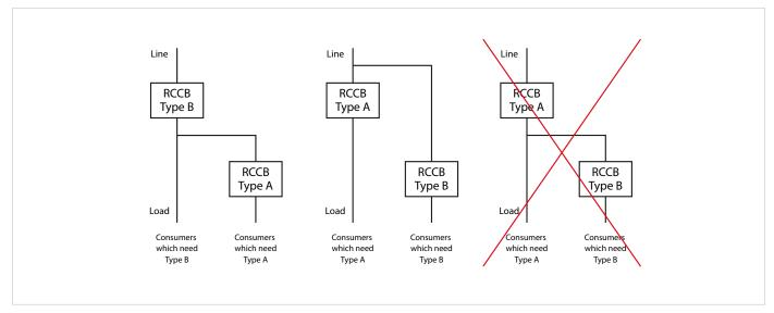
Fig. 9: Permissible and non-permissible RCD Type A/Type B scenarios
