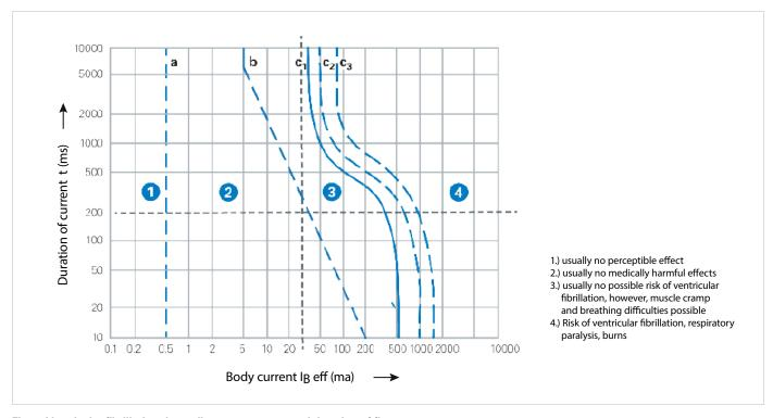
Fig. 1: Ventricular fibrillation depending on amperage and duration of flow
