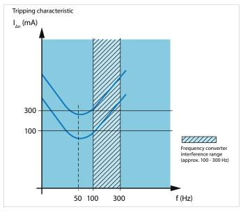
Fig. 5: Type U RCD tripping characteristic
