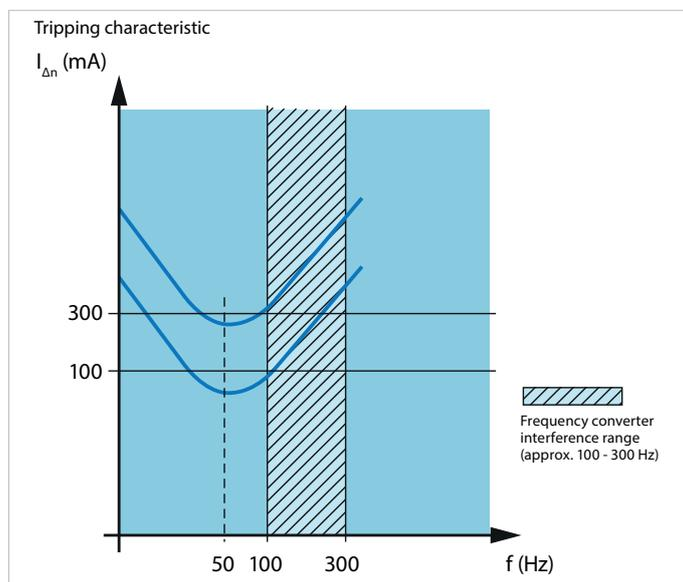
**Fig. 5: Type U RCD tripping characteristic**
