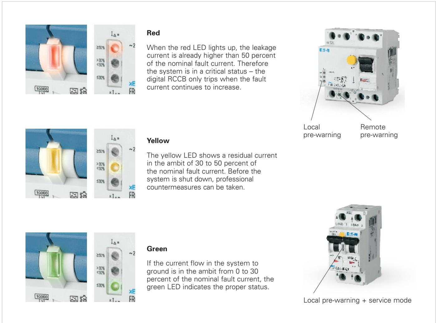
Fig. 7: Digital RCDs alert maintenance staff of problems before a blackout occurs
