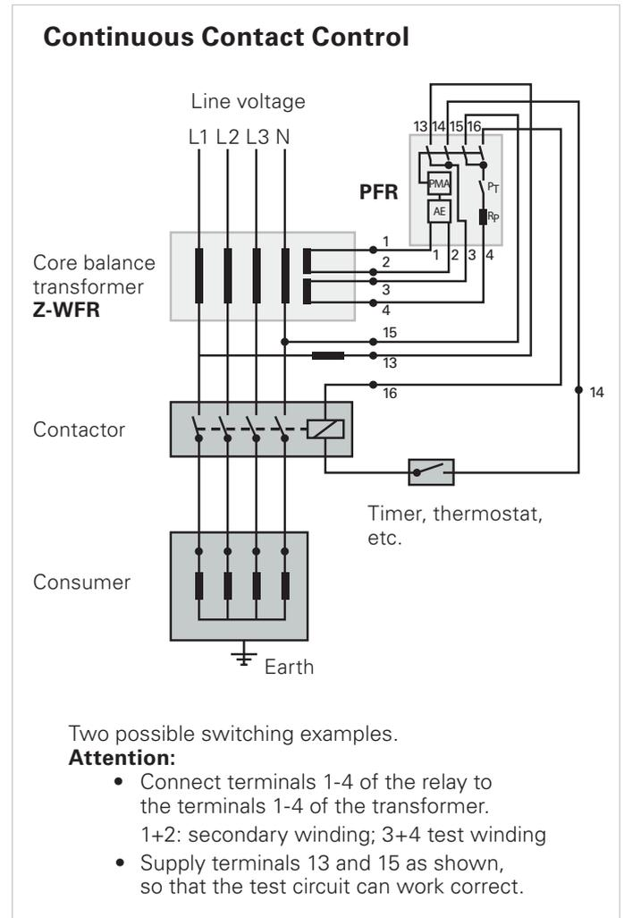
**Fig. 6: RCD relay switching example**
