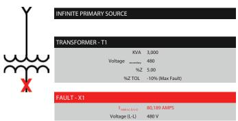
Short-circuit current is calculated on the transformer secondary assuming infinite available short circuit-current on the primary.
