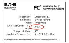
Elevator control panel has a manufacturer's nameplate SCCR of 10 kA and is field marked with available short-circuit current 9055 A.
