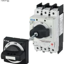
Eaton door mounted rotary and supplementary handle kits comply with all the requirements of the UL 508A and NFPA 79 standards with respect to the operating handles of supply circuit disconnecting switches for industrial machinery, including a deliberate action design incorporated into the supplementary handle to meet the enclosure interlocking provisions of the standards.
