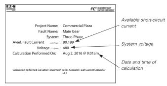
Bussmann series FC<sup>2</sup> available fault current calculator produces label images of the available short-circuit current calculation for field marking equipment.
