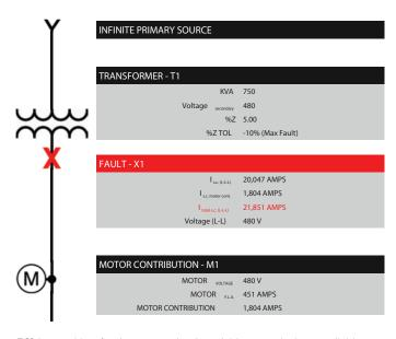
FC<sup>2</sup> is capable of using many circuit variables to calculate available short-circuit current, including motor contribution.
