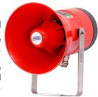
cULus and ATEX dual certified, 12-48Vdc, corrosion resistant GRP explosion proof enclosure with a red rugged thermoplastic flare, 2 x 1/2" NPT cable entries with a certified zinc plated steel plug fitted, 112dB sound output @ 10 feet.
